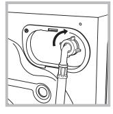
1. Connect the inlet hose to the machine by screwing it onto the cold water inlet of the appliance, which is situated on the top righthand side of the rear part of the appliance (see figure).
